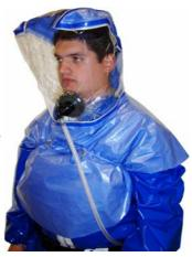
The 360° swivelling airline system mounted on an adjustable belt incorporates a hose restraint fitting and an audible low flow warning device. The lightweight soft elasticated neck seal is designed for comfort and to permit removal of a contaminated hood without touching the inner surfaces.
