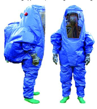
Laminated anti-mist visor giving clear undistorted vision. Single valve to side of hood to ensure that the pressure change within the suit does not exceed 4mbar. 117cm (46") Fine tooth zip fitted to rear of suit, closing at bottom complete with single storm flap with double-sided tape. Permanently attached highly chemically resistant laminated gloves (welded).
